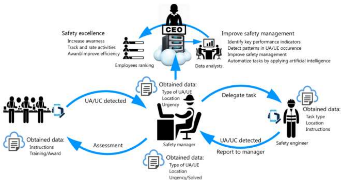
Figure 1 – The generic workflow of an arbitrary Safety 4.0 reporting solution as defined in Vukicevic et al. 2019 [11]
